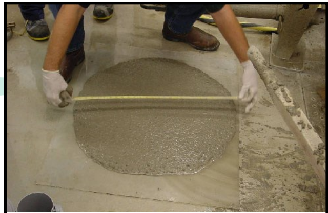
Measuring Slump Flow of SCC
